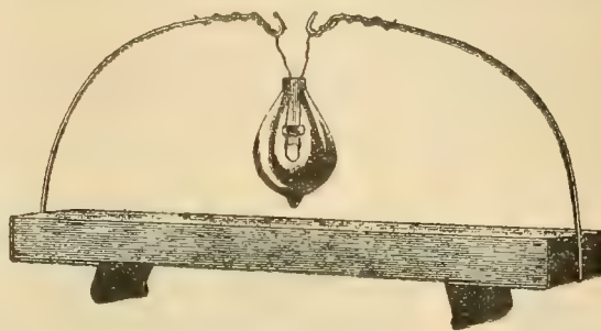
FIG. 4.—INCANDESCENT LAMP ARRANGED FOR PROJECTION.
